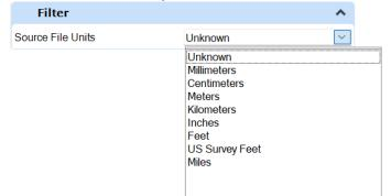
C. .The NCDOT Seed File uses US Survey Feet, if the source data were in Meters or Miles the user could specify those units and the import process could convert the data to US Survey Feet
