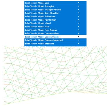
J. Turn off the *Exist Terrain Model Triangles* and all the elements will turn off. This is because the Triangles are the actual surface. Like many other civil elements in ORD the surface is a dynamic element and without the triangles displayed the elements in the surface; contours, breaklines, boundaries etc. cannot be displayed.
