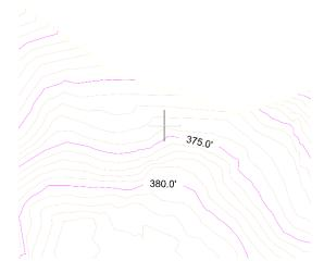
F. Snap to the location of an element that will be the center of rotation. In this example snap to a point on one of the contour lines. Left click to set the rotation at that location. It is important to snap to an element to set the Z elevation correctly for the rotation point.
