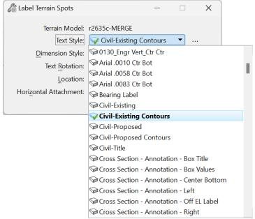
D. Set the Dimension Style to <a>Lbl-RDY-Pln\_Terrain Spot Elevations</a>
