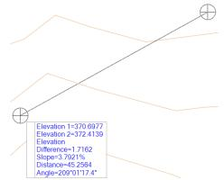
F. Select the second point left clicking inside the terrain model boundary. A line will be drawn in the dgn file that shows the location of the two points and a dialog will appear that shows the relevant elevation and slope data based on those two points.
