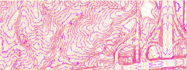
10. By attaching the original R2635C\_RDY\_ETM.dgn file the user can see the overlap of the LIDAR data and the survey data near the first interchange. This LIDAR dataset will be used in later exercises to demonstrate merging and clipping operations.
