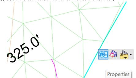
N. Select the Properties Icon from the context menu, note that the individual components of the Terrain model are Grayed out.
