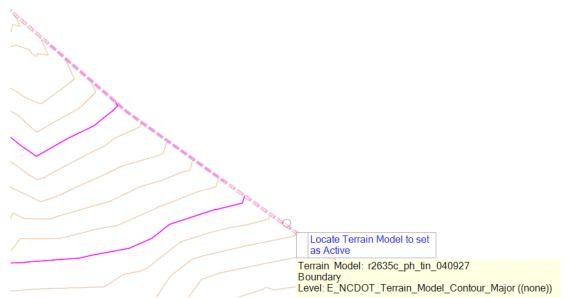
18. The process of creating the ETM file that will be used throughout the project is now complete. There are no additional steps required to begin using the surface to design profiles and models or create cross sections and develop quantities.
